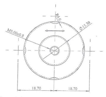
Note: Unspecified linear tolerance is ±0.05 Angular tolerance is ± 0°15'
